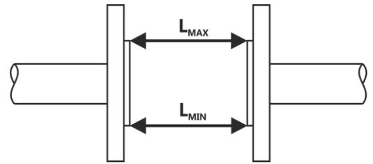
The opposition of the holes in the counter-flanges for the bolts should be ensured in the same manner and a sufficient room behind the flanges should be available for the bolts and nuts so that the actual installation of the sensor in pipeline and its attachment with the bolts is made possible.
