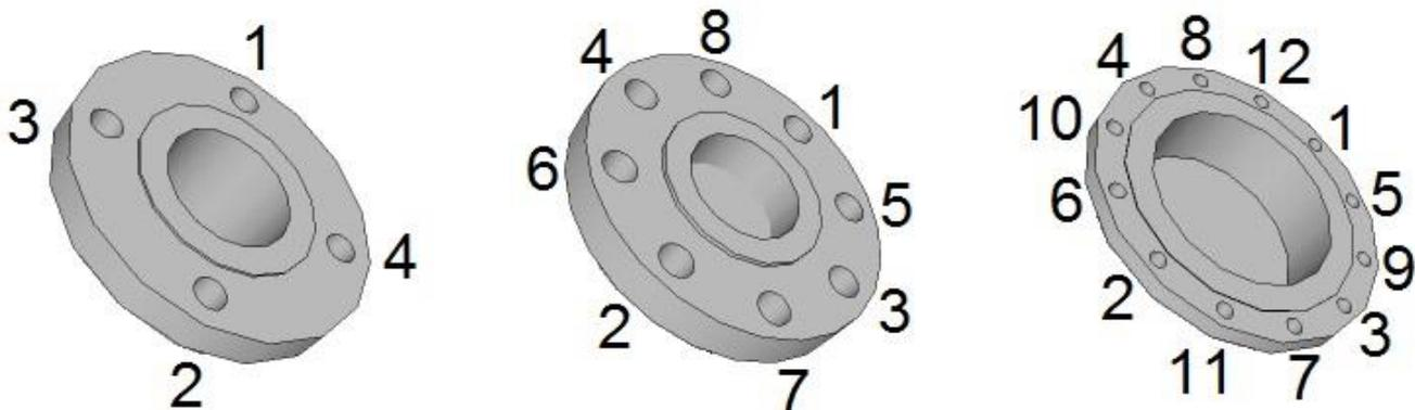
If the bolts are tightened too much during the installation of pipework components, deformation of the sealing surface may occur. In consequence, the torque values indicated in the table are used as a guidance for tightening the screws and bolts.
