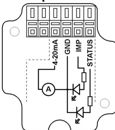
The maximum frequency of the pulse output is 1,6kHz when pulse width min. 250 $\mu$ s
