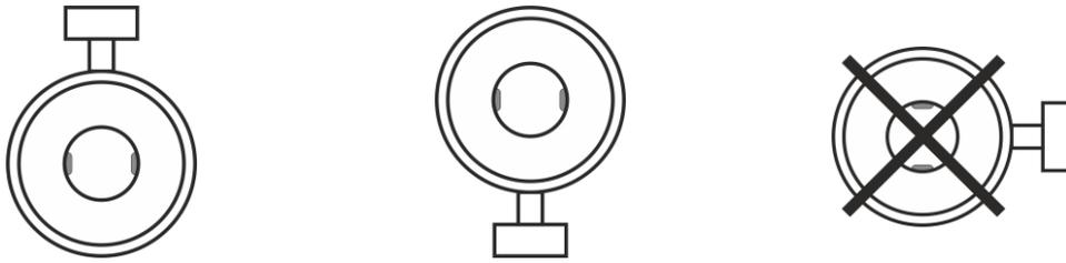
2) in the version with earthed electrode and/or empty piping test electrode (3/4 of the electrode)
